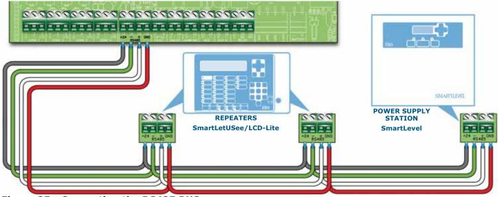
Figure 25 - Connecting the RS485 BUS
