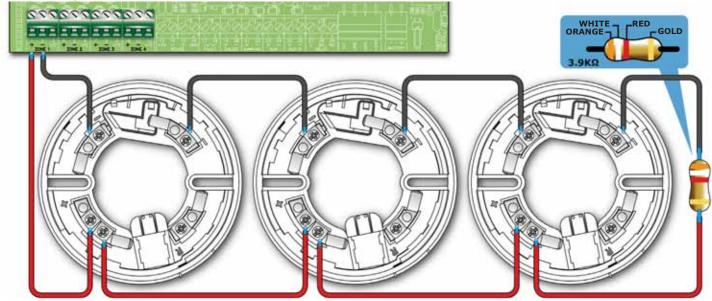
Figure 14 - Connecting Iris detectors
