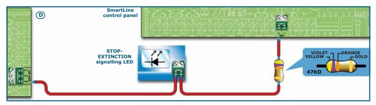
Figure 32 - Extinguishant module
