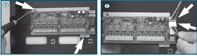
Figure 11 - Mounting the expansion board - 1
