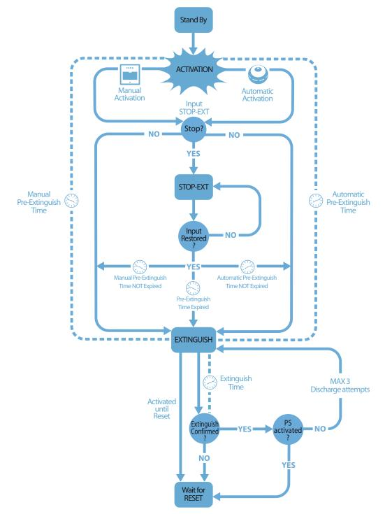
Figure 36 - Extinguishant board: operating principles
