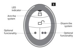
NOTE: Fig. No. 1 reflects the default EWK2 button configuration. All keyfob buttons are configurable according to individual needs.
