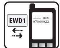
Here "ID1" means magnetic door contact identification number. This identification number can be found on the back of the device. The system automatically provides two security zones to the connected door contact. The system informs about this via SMS message, for example, "ID1:Z14:ID1Z15" - here instead of "ID1" will be identification number of the module that you want to connect, "Z14 and Z15" – the numbers of free zones provided by the system.
