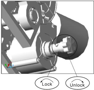
When unlocking the boom could suddenly move upwards. Always control the boom movement with your hands.
