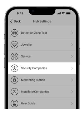
The list of organizations connecting the Ajax system to the central monitoring station is provided in the **Security Companies** menu of the hub settings:
