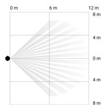
Horizontal viewing angle of the detector
