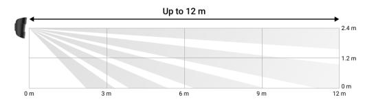
Vertical viewing angle of the detector
