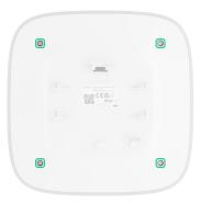
**4.** Turn the siren over while holding the front and back of the body. Remove the protective plastic panel.
