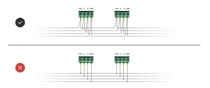
**+24V** — power phase **A, B** — signal terminals **GND** — ground
