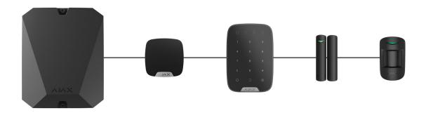
For the **Beam (Radial)** topology, be sure to install a 120 Ohm terminating resistor at the end of the line (included in the hub complete set). The terminating resistor is connected to the signal terminals of the last device on the line.
