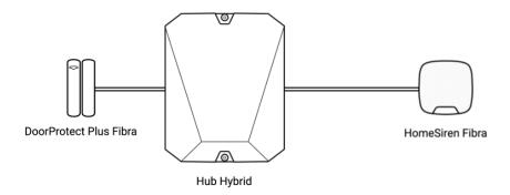
DoorProtect Plus Fibra is a wired opening, shock, and tilt detector. It connects to the hub via a metallic bus and uses Fibra protocol.
