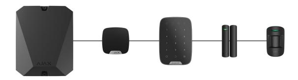
For the **Beam (Radial)** topology, be sure to install a 120 Ohm terminating resistor at the end of the line (included in the hub complete set). The terminating resistor is connected to the signal terminals of the last device in the line.
