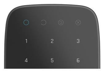
KeyPad Fibra can report the current security mode, button pressings, malfunctions, and other conditions with LED indication and a sound signal.
