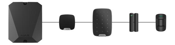
**Ring connection method** occupies two Fibra lines of the hub. If the ring breaks in one place, no device will be disabled. The ring reconfigures into two lines, which continue to operate normally. Users and the security company will receive notification about the break.
