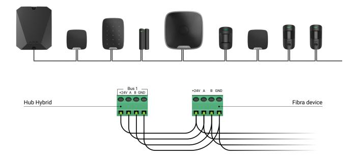
For the **Beam** (**Radial**) topology, be sure to install a 120 Ohm terminating resistor at the end of the line (included in the hub complete set). The terminating resistor is connected to the signal terminals of the last detector on the line.
