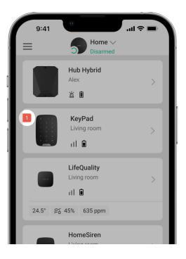
If a keypad malfunction is detected, a malfunction counter is displayed in Ajax apps in the upper left corner of the device icon.
