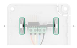
3. Prepare holes for cable output in advance. To output cables from the back of the keypad, break out the perforated part on the SmartBracket mounting panel. To output cables from the bottom of the keypad, make holes in the bottom of the enclosure using a drill bit, a special milling cutter for small holes, or handcutting tools.
