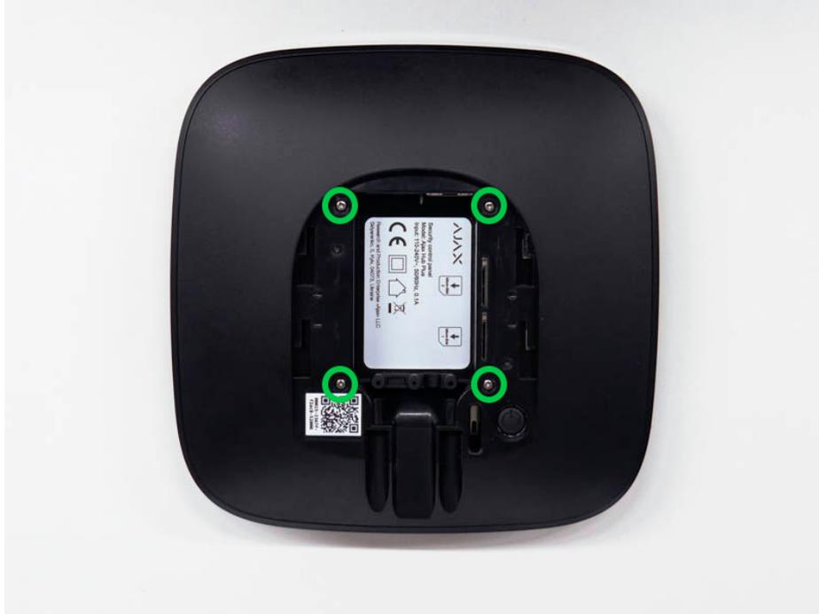
5. Remove the screws attaching the boards to the device body.
