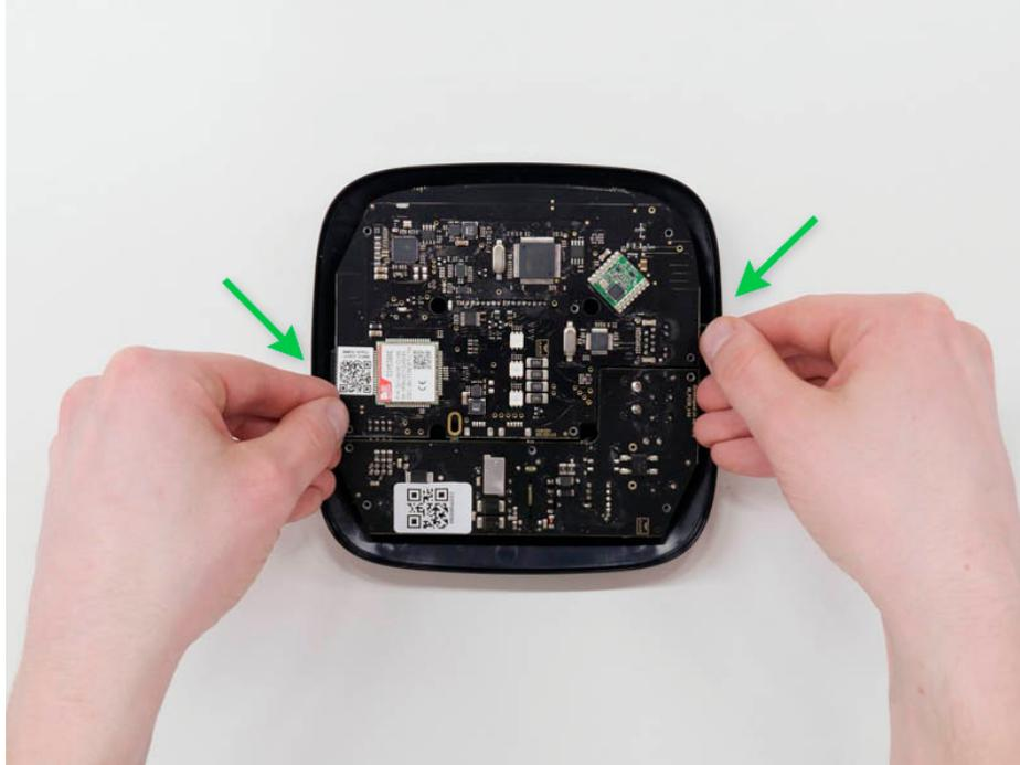
7. Disconnect the power supply unit (smaller board) from the mainboard.
