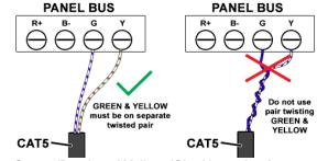
Note: Green (Data) and Yellow (Clock) need to be on separate pairs otherwise bus errors will occur.
