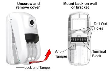
If you are installing the HD88 near any reflecting surface, please note that it may affect the quality of the night vision due to the IR reflection.
