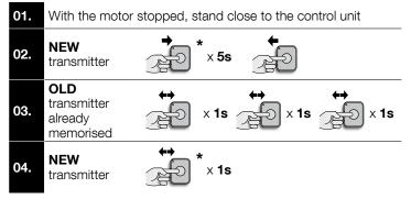
If the procedure terminated successfully the new transmitter is mem-
