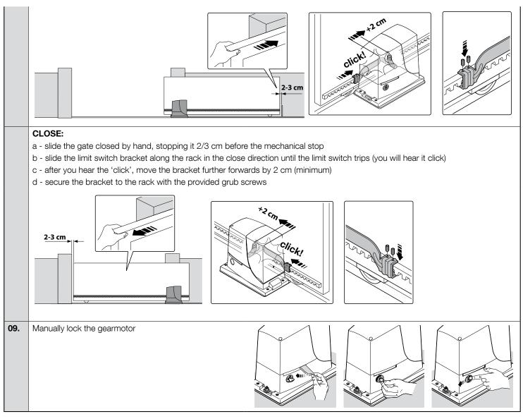
Manually lock the gearmotor.
