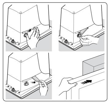
Manually locking the gearmotor
