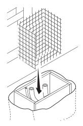
Insert the screws supplied in the anchoring plate. Lock the screws in place with the nuts supplied. Remove the pre-shaped clamps using a screwdriver. Fit the anchoring plate in the iron cage.
