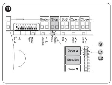
LEDs "L1" and "L2" on the control unit ("Figure 11") emit some slow flashes to signal that the learning procedure must be carried out.
