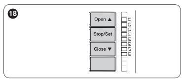
The available programmable functions are grouped into **two levels** and their operating status is signalled by eight LEDs "L1 ... L8" located on the control unit (LED lit = function enabled; LED off = function disabled).
