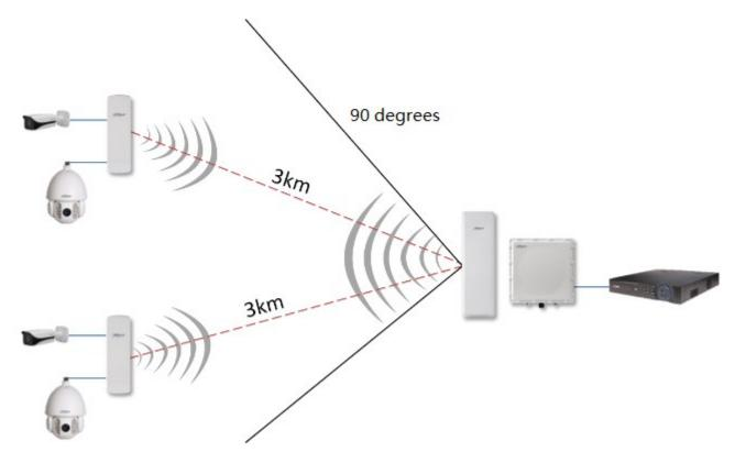
Figure 3-2 Point-to-multipoint Networking Diagram
