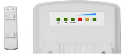
Figure 1-1 LED Indicator Light on DH-PFM881 Shell
