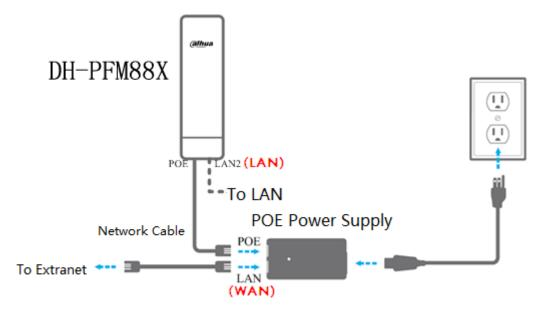
Figure 7-1 Connection Diagram of Route Mode
