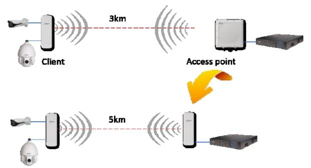
Figure 3-1 Networking Diagram of Access Point and Client
