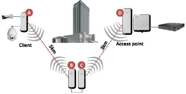
Figure 3-3 Networking Diagram of Coverage Dead Angle Adjustment
