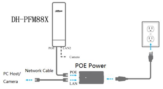
Figure 2-4 DH-PFM88X Interface Connection Diagram
