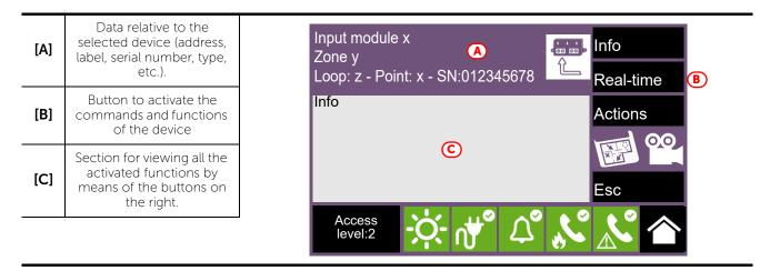
The function buttons [B] that operate on the device vary depending on the type of device shown or the user access level:
