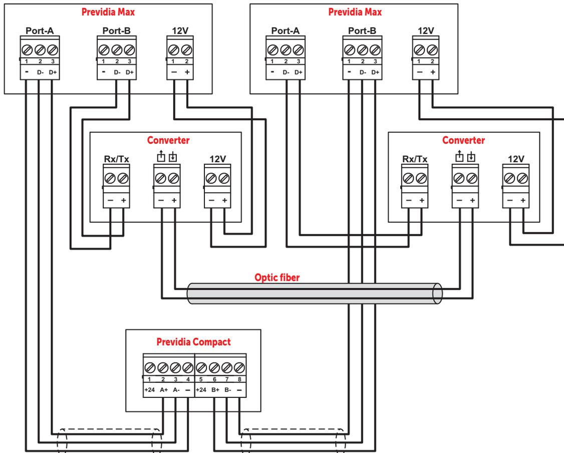
In cases where a fiber optic cable is used over long BUS lengths, it is necessary to use a RS485/fiber converter (non-INIM brand product). The module IFMNET has a 12V output (*paragraph 3.1 - [C]*) for the power supply to the converter in use.
