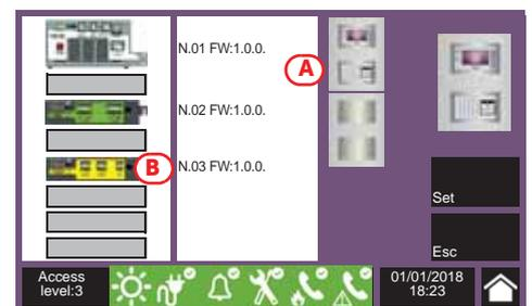
**for Previdia Compact:** Access to control panel programming and press the **Configuration** button. In the configuration section, touch the networking programming access icon.
