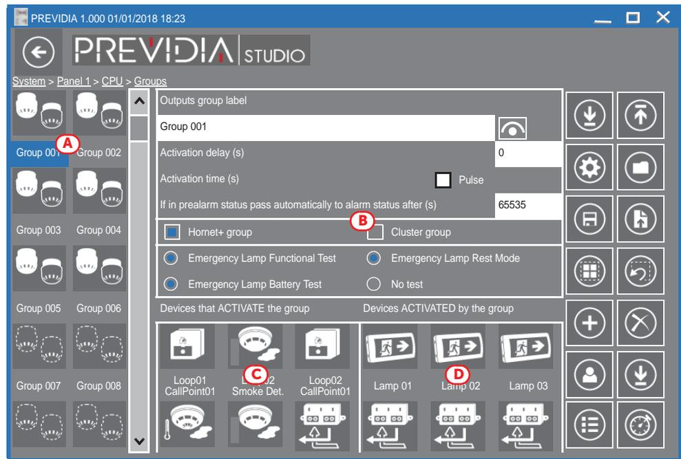
Once the **Hornet+ group** option is activated, in the parameters section of the selected group (*B*), the group will be the same for all the control panels in Hornet+ network. The outputs associated with the group will activate regardless of control panel they are connected to. In the same way, the devices of any network control panel can activate the shared group.
