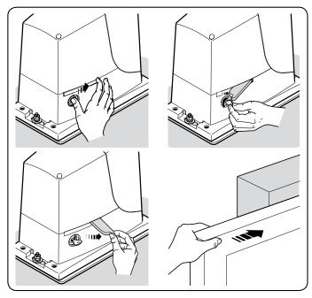
Manually locking the gearmotor
