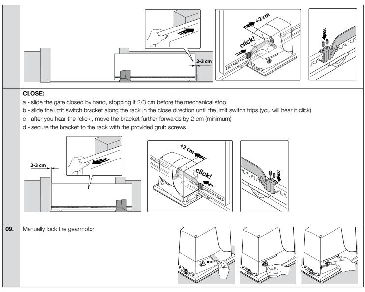
Manually lock the gearmotor.
