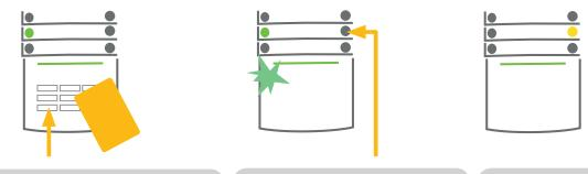
**1. Authorize** yourself using the keypad (enter a code or hold a card or tag up to the reader). The green backlit indication button will start flashing.
