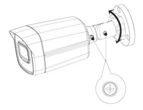
Figure 3-27 Model L adjustment
