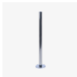
Galvanized steel post with fastening flange and chromed-plastic flange cover. H = 980 mm. Available without holes, with 2 holes, with 2 + 2 holes at 90° or at 180°, with 6 holes, and with 8 holes.
