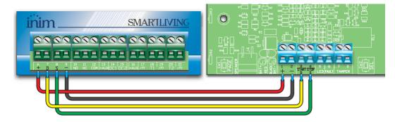
Connection of the LED terminal to an open-collector output, will allow management of the STATUS and PRG LEDs, flasher and horn directly from the intrusion-control panel (as programmed).
