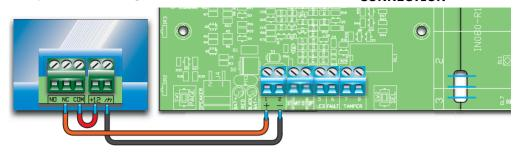
This wiring method activates signaling via the START terminal and deactivates it via the STOP terminal. The polarity of both inputs is programmable.
