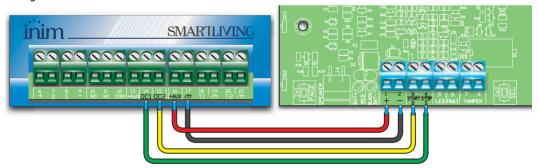
Only the Ivy-B, Ivy-BF, Ivy-BM and Ivy-BFM models can be **I-BUS** connected to the I-BUS wire. This connection allows you to program the device and activate alarm-signaling directly from the panel.
