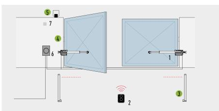
1. MOTOR 2. TRANSMITTER **3.** POST-MOUNTED PHOTOCELLS 4. PHOTOCELLS 5. FLASHING LIGHT 6. CONTROL UNIT 7. DIGITAL OR KEY SWITCH
