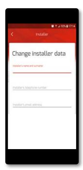
You can enter the name and references of your installer in the U-control app. In case of a system failure, the installer can be contacted directly from the U-control app, emailing also the last error detected by the central unit
