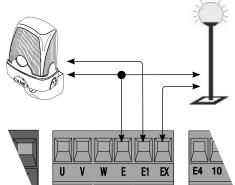
Cycle/courtesy lamp (Contact capacity: 230 V - 60 W max.).
