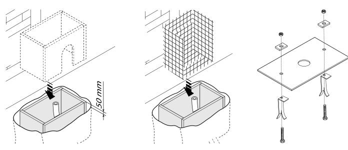
Position the mounting plate, respecting the measurements shown on the drawing, if the rack is already present. Caution! The tube must pass through the prepared hole.
