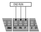
If installing on the right, inside view, reverse the motor and end run terminals on the control panel.
