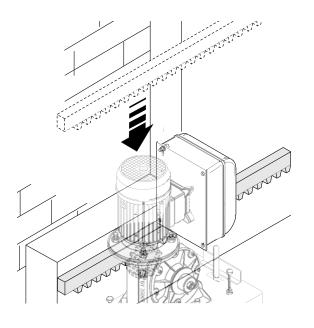
Weld or secure the rack to the gate along its entire length.
