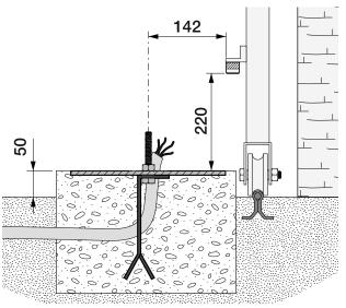
Fill the counterframe with cement. The plate must be perfectly level with the screw threads completely on the surface. Allow to cure for at least.
