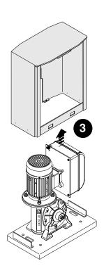
Position the gearmotor above the mounting plate. Caution! The electrical cables must pass under the gearmotor box.
