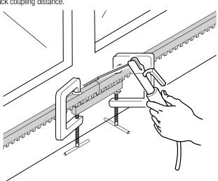
Open and close the gate manually and adjust the pinion/rack coupling distance using the threaded feet (vertical adjustment) and the slots (horizontal adjustment). This prevents the weight of the gate bearing upon the operator.
