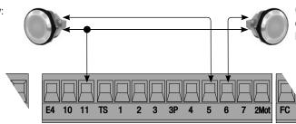
Gate closed indicator light (contact capacity: 24 V - 3 W max.) Indicates that the gate is closed.
