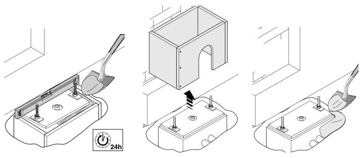
Remove the nuts and washers from the screws.
