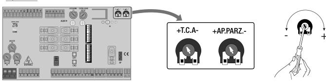
ACT trimmer - Adjustment of the AUTOMATIC CLOSING time: from a minimum of 1 second to a maximum of 120 seconds.
