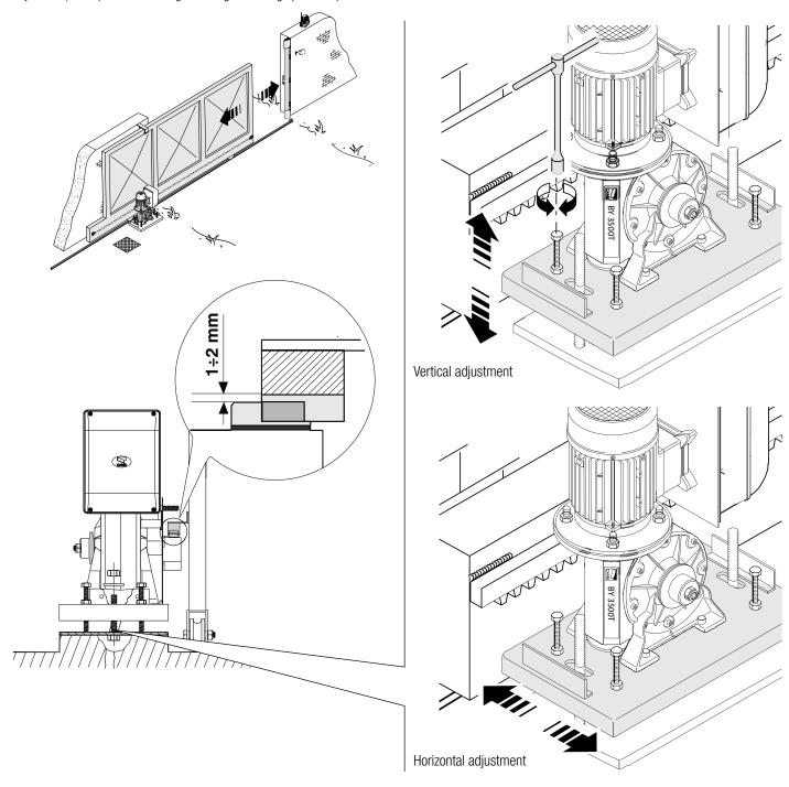
When adjustment is complete, secure the gearmotor to the plate using the washers and nuts.
