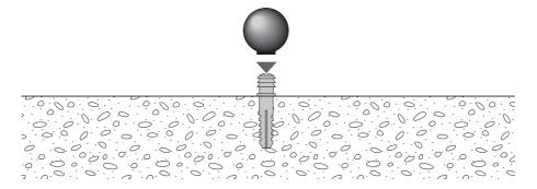
Fix the end stop to the ground so it acts as a mechanical opening stop.
