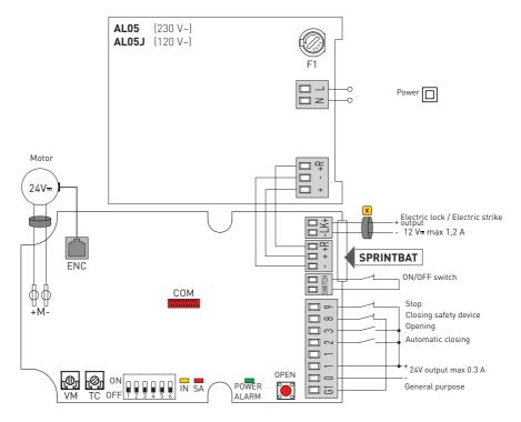
Install the ferrites (supplied) in the point indicated by the  $\boldsymbol{X}$ , as shown in the figure
