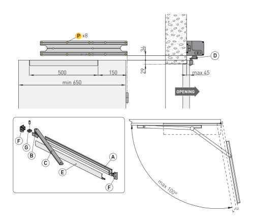
Use the SBS sliding arm for doors that open inwards (as seen from the automation side).
