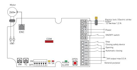
Where there is an X, install the ferrites supplied (as shown in the figure)
