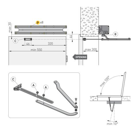
Use the SBA articulated arm for doors that open outwards (as seen from the automation side).
