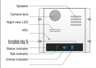
**Note:** Key A and key B can not be seen on the panel, they are cryptic. Normally, key A and key B are not active. **To activate the buttons, just set the DIP6 to ON position**
