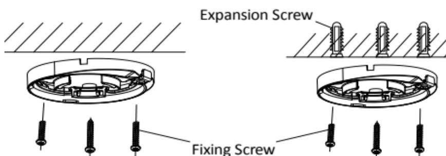
Figure 2-8 Fix the Mounting Base to the Ceiling
