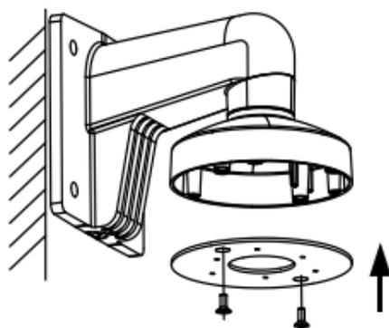
Figure 2-14 Install the Adapter to the Pendent Cap
