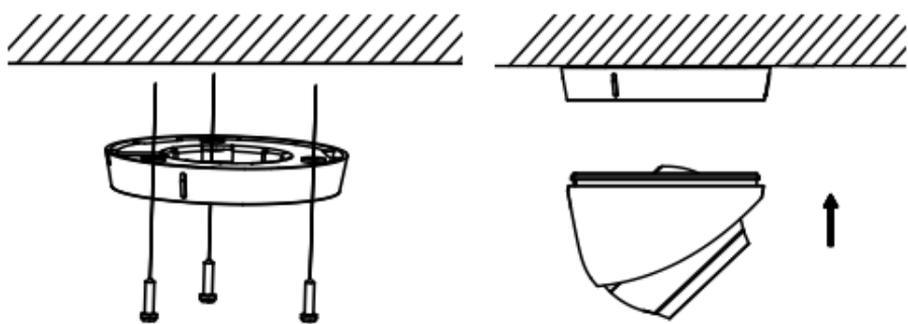
Figure 2-3 Fix the Mounting Base and Camera
