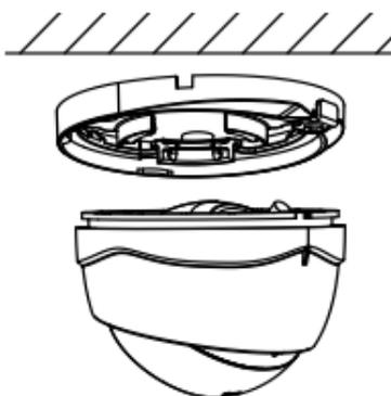
Figure 2-9 Secure the Camera
