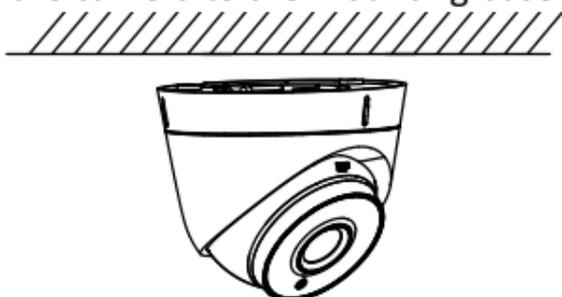
Figure 2-4 Fix the Camera to the Ceiling
