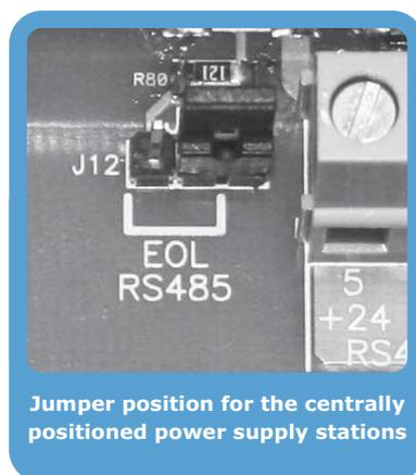
Figure 27 - SmartLevel board - jumper position
