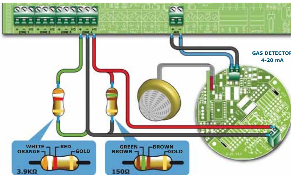
**Figure 21 - Connecting 4-20 mA gas detectors**
