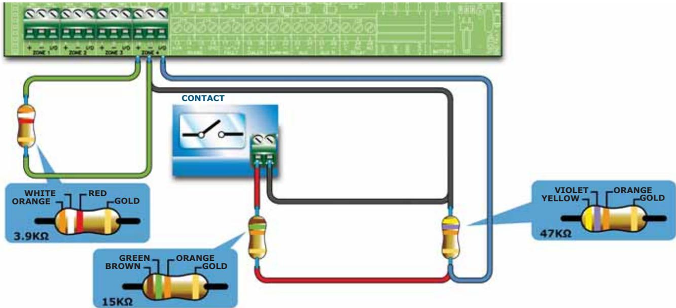
**Figure 20 - Wiring the I/O line as an input**
