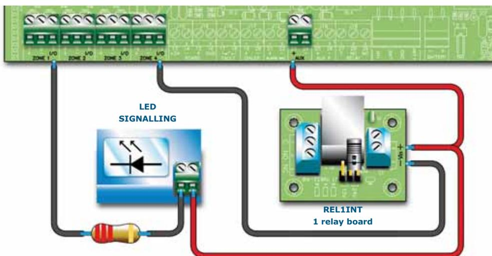
**Figure 19 - Wiring the I/O line as an output**
