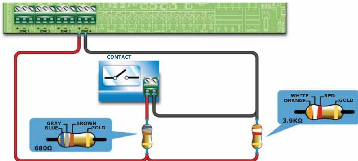
**Figure 18 - Connecting generic contacts to the detection line**
