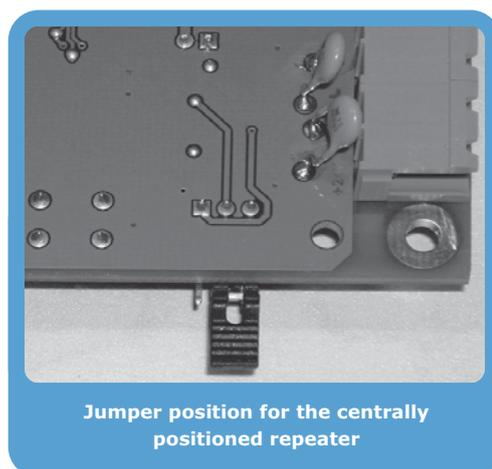
Figure 26 - SmartLetUSee/LCD-Lite board - jumper position
