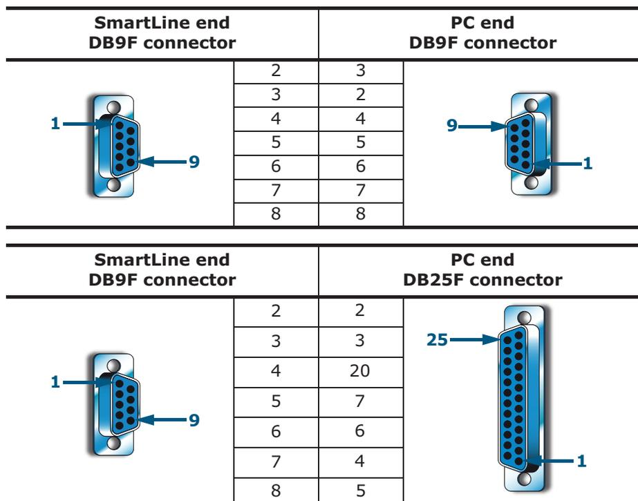
**Note:** The RS232 link can be ordered separately. The order code is indicated in Appendix B - Order codes. If your PC does not have a RS232 port but has a USB, use an RS232-USB adapter.
