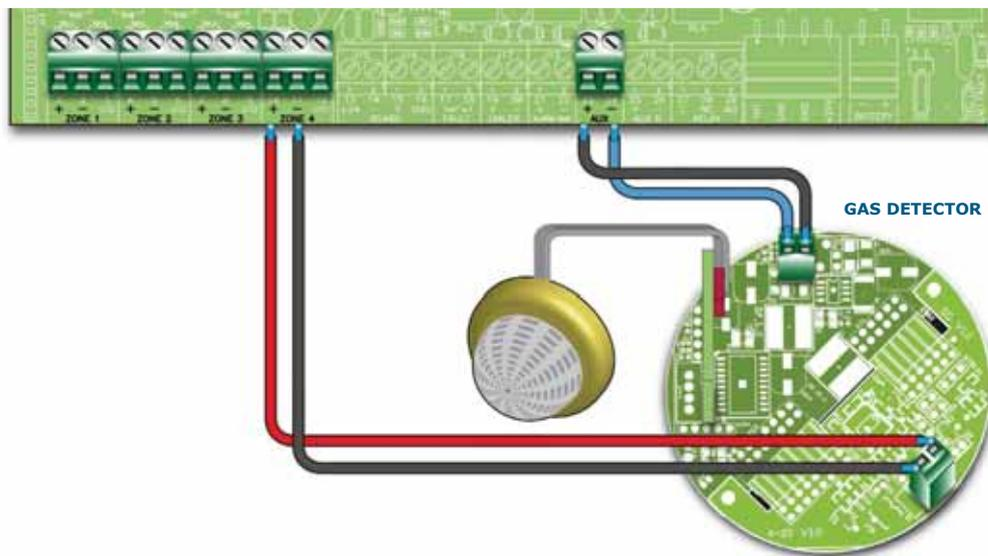
**Figure 17 - Connecting gas detectors to the detection line**
