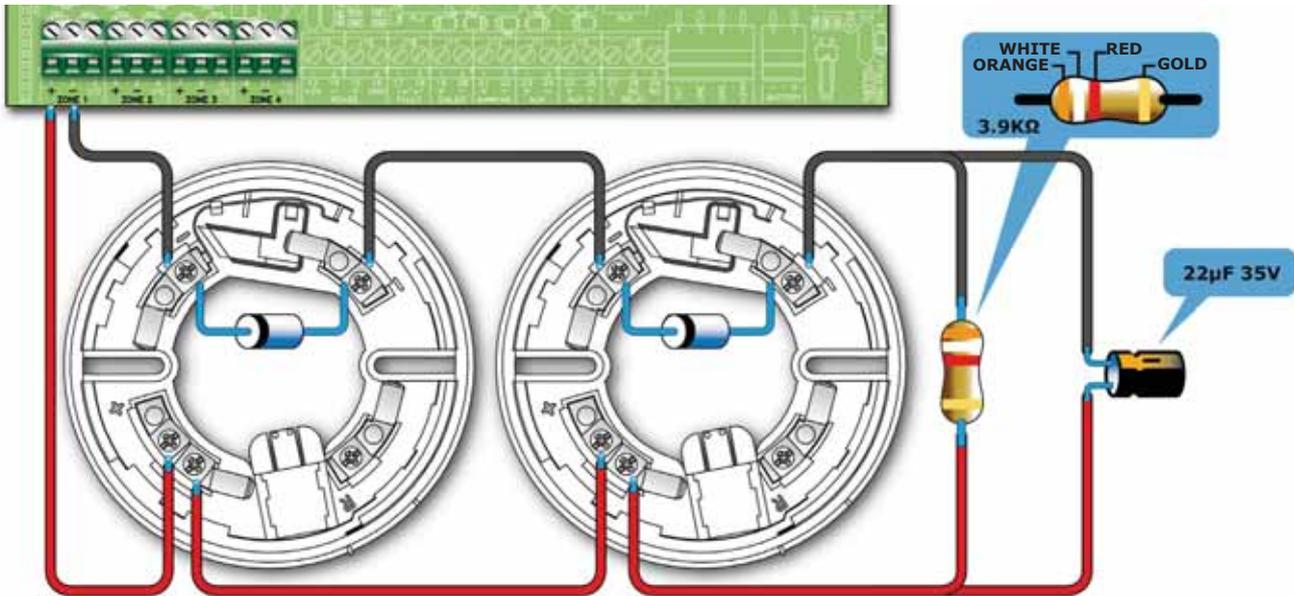
**Figure 16 - Wiring for detection with missing detectors**
