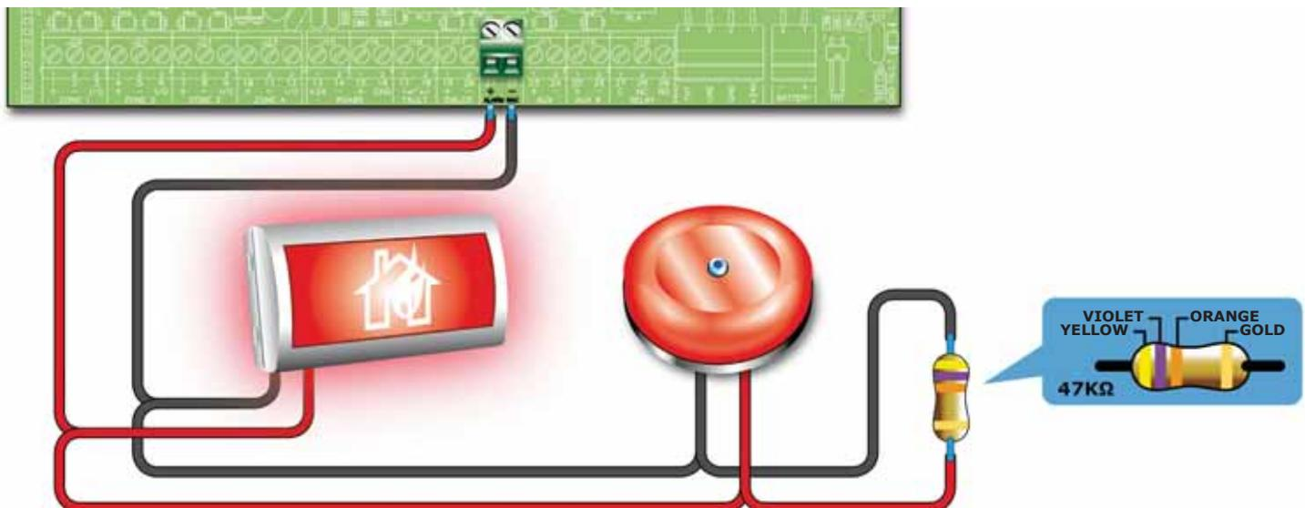
**Figure 29 - Connecting the Alarm output**
