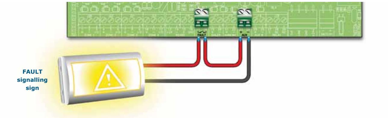
**Figure 28 - Connecting the fault signal output**
