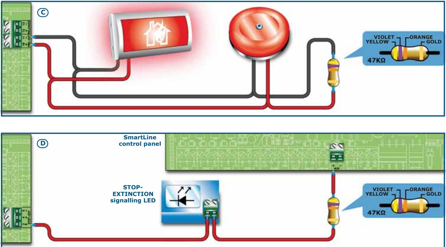
Figure 32 - Extinguishant module
