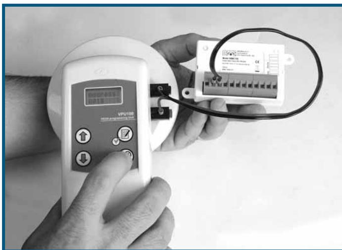
**Figure 34 - Addressing modules using a VPU100**
