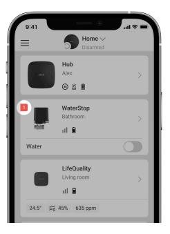
If a malfunction is detected in Ajax WaterStop (for example, there is no connection with the hub or range extender), the malfunction counter is displayed in the device field in Ajax app.
