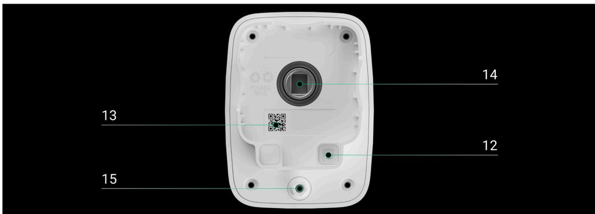
12. Tamper button. Reacts to the removal of the electric actuator from the mount.
