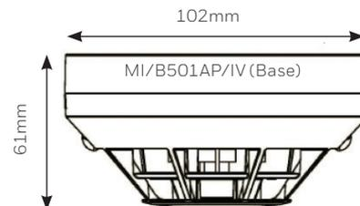
The optical-thermal detector conforms to EN54-7, a 58°C fixed temperature and rate of rise thermal assistance conforming to EN54-5. The thermal detection function combines thermistor technology with a software corrected linear temperature response. In areas where the normal daytime activities may potentially create unwanted alarms, the detector can be programmed to operate in a “heat only” mode, automatically reverting to full photo-thermal operation during unoccupied periods.
