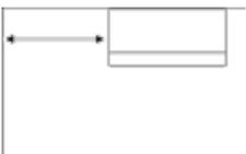
Moreover, if the control unit must be installed to the wall beside a corner wall, the minimum distance from the latter must be at least 200 mm, so as to avoid the opening of the front panel.
