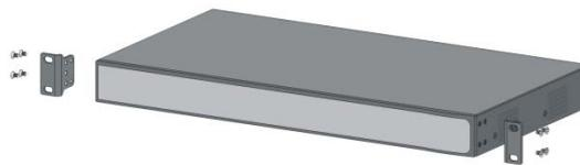
Step 3 Fix the Device to the rack with screws.
