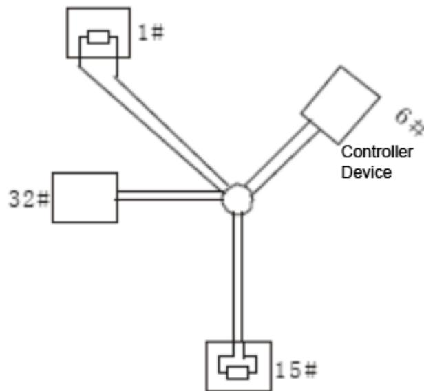
To fix the issues, it is recommended to use RS-485 distributors. The RS-485 distributor can help avoid the common connection issues so as to improve transmission quality.
