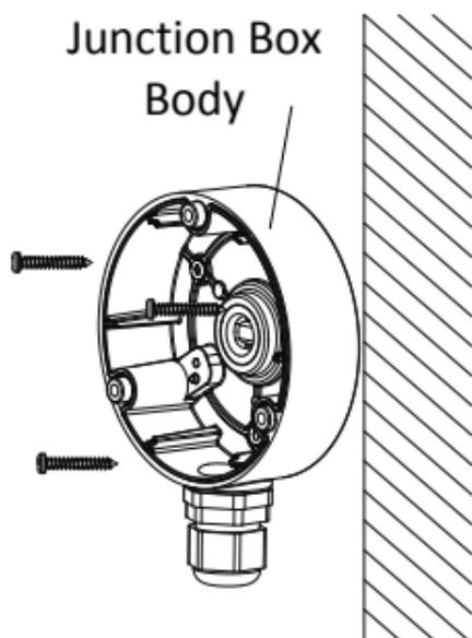
Figure 2-4 Secure the Junction Box on the Wall/Ceiling
