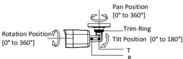
Figure 2-2 3-Axis Adjustment
