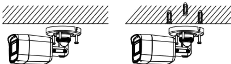
Figure 2-1 Attach the Camera to the Ceiling
