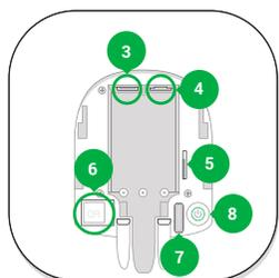
3 - Socket for connecting a power supply cable.
