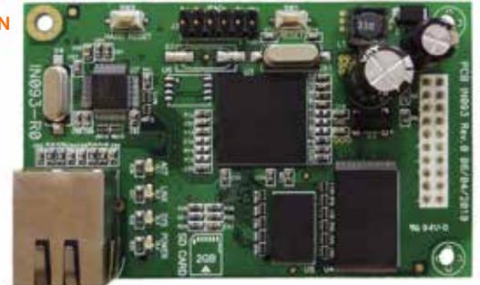
The SmartLAN board is capable of sending detailed e-mails for each event and real-time event reports via TCP/IP. The board provides a web server for access to the control panel via web without any proprietary app.
