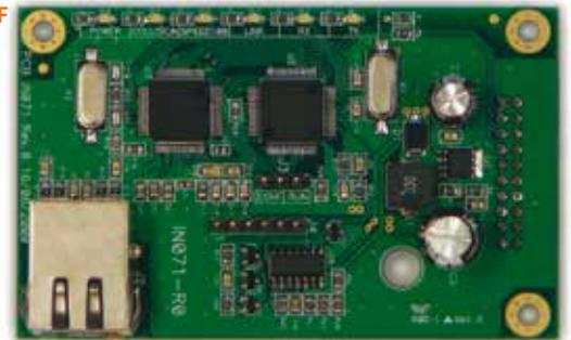
The SmartLAN and SmartLAN/SF boards connect to any Ethernet network and allow remote access (via Internet) to the control panel and to all control panels present in the HorNet network. These boards also allow remote programming (upload/download operations) and remote system monitoring via the SmartLook supervisory application.
