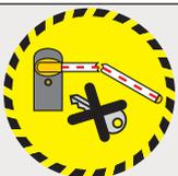
⚠ **WARNING!** This release procedure is potentially hazardous for users, when for whatever reason, such as the boom being badly fastened, ripped out or broken during an accident, and so on, the loosened springs no longer provide the proper balancing action. This could lead to a sudden rotation of the boom attachment and/or of the boom itself.
