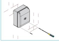
2) Perforate the marked holes and insert the cable glands with corrugated tubes for the electrical cables to run through.
