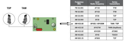
Plug in the radio-frequency card onto the electronic board AFTER CUTTING OFF THE MAIN POWER SUPPLY (and disconnecting the emergency batteries).
