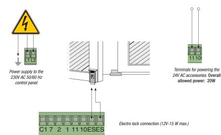
Flashing light (contact rated for: 230V AC - 25W Max.) Flashes while gate opens and closes.
