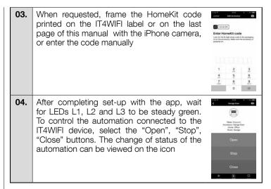
▲ If the procedure described does not terminate successfully, check that the requirements indicated at the beginning of the manual are satisfied, run the IT4WIFI Reset procedure using the P button (Chapter 8) and then try again.
